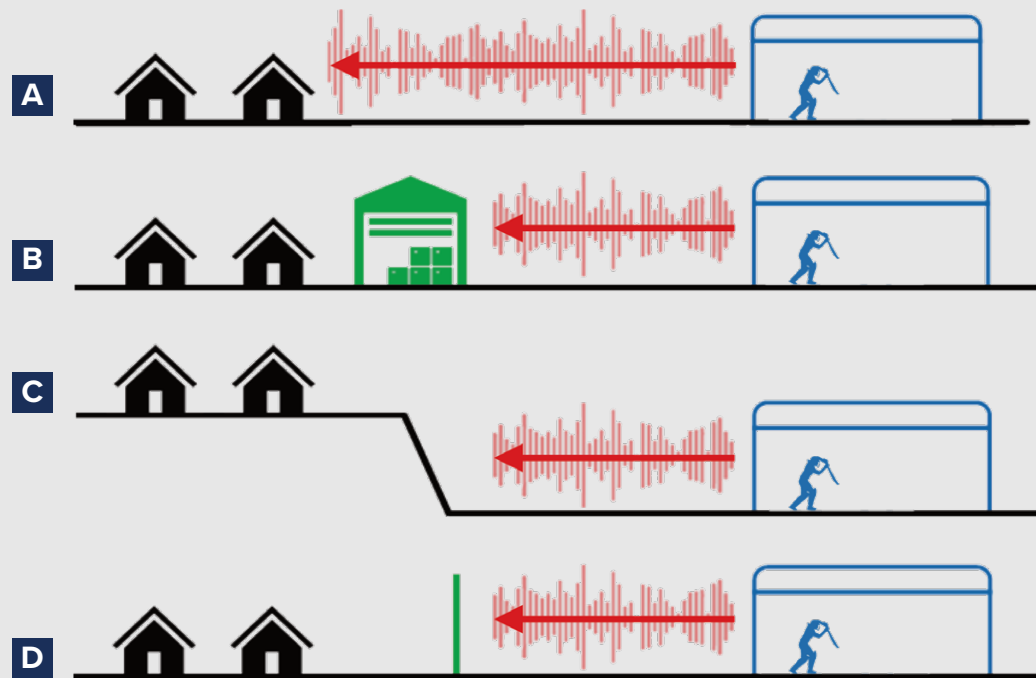
Figure 39. Example noise mitigation strategies for a Covered Outdoor Cricket Facility. A - unacceptable noise breakout adversely impacting upon neighbouring noise sensitive receivers. B - acceptable noise breakout where a non-sensitive building forms an acoustic screen to neighbouring noise sensitive receivers. C - Acceptable noise breakout where topographical features form an acoustic screen to neighbouring noise sensitive receivers. D - Acceptable noise breakout where a proprietary acoustic fence forms a screen to neighbouring noise sensitive receivers.
